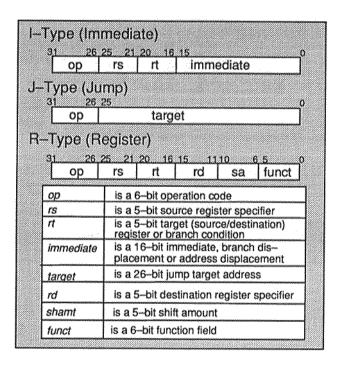
In addition to the standard R2000 formats shown above, the MIPS-lite instruction set also has an additional format for the BLTZ and BGEZ instructions.
